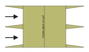
**Step 4:** Fold the legs of the cover inwards so that it lays on top of the roof
