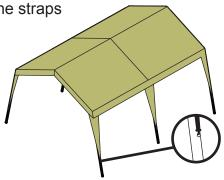
**Step 6:** To secure the gazebo hammer the stakes into the ground then and secure the guy ropes to the stakes
