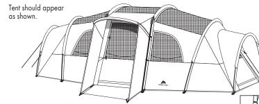
STEP 15: Unfold fly and place over tent. Attach the hooks on the fly corners to the metal rings on the main upright poles and the fabric loops on the side room pole sleeves.
